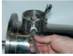
Guide cable through the cable gland into the terminal box. Ensure that the assembly and fastening of gland is carried out carefully in order to maintain the protection class, if necessary use additional compound material for the thread. Should the second cable entry not be used, this must be thoroughly closed with the blind plug out of stainless steel.
