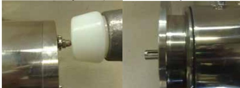
Attention: By no means should one try to open the motor with a screw driver or the like, in the joint between shield and housing.
