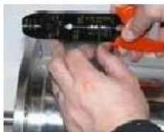
Properly remove the insulation from the motor leads and the cable leads and have a shrink hose ready with a corresponding diameter and length.
