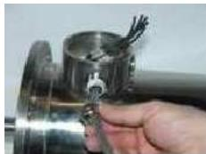
Guide cable through the cable gland into the terminal box. Ensure that the assembly and fastening of gland is carried out carefully in order to maintain the protection class, if necessary use additional compound material for the thread. Should the second cable entry not be used, this must be thoroughly closed with the blind plug out of stainless steel.
