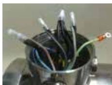
Connect motor leads and cable leads with suitable crimp connectors acc. to the connection diagram. The same applies to the PTC thermistors if necessary.
