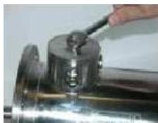
Open the cover of the terminal box with suitable tools.
